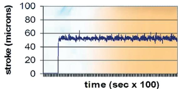
NO consistency between the programmed phaco tip stroke and the actual tip elongation, when the phaco tip faces the resistance presented by hard lens material.\*
